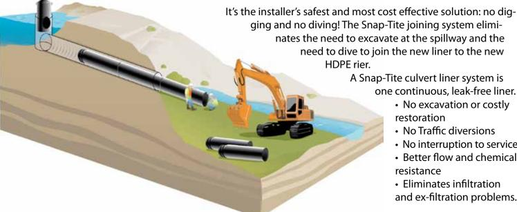
A Snap-Tite culvert liner system is one continuous, leak-free liner.
