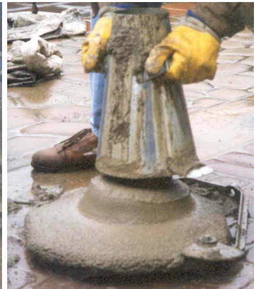
Mix after the addition of AERFLOW™ with slump of 7-9 in
