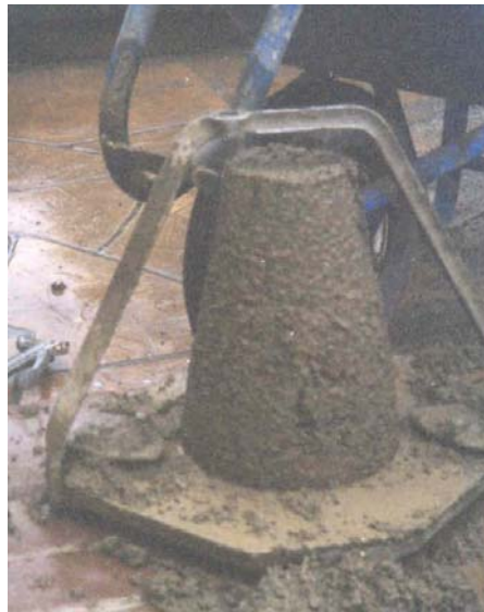
Initial Mix with 1.5 in slump, before addition of AERFLOW™
